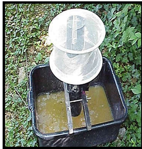
Gravid traps are intended primarily to monitor Culex mosquito populations
